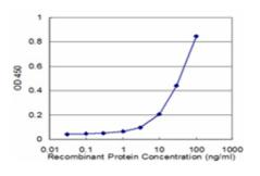
Detection limit for recombinant GST tagged MPP1 is approximately 1ng/ml as a capture antibody.
