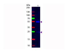
Western Blot of Mouse anti-Goat IgG Fluorescein Conjugated Secondary Antibody. Lane 1: Goat IgG. Lane 2: None. Load: 50 ng per lane. Primary antibody: None. Secondary antibody: Fluorescein goat secondary antibody at 1:1,000 for 60 min at RT. Block: MB-070 for 30 min at RT. Predicted/Observed size: 25 & 55 kDa, 25 & 55 kDa for Goat IgG. Other band(s): None.
