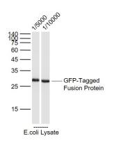
Sample: GFP-Tagged Fusion Protein Overexpression E.coli Lysate (Cat#: bs-33009P) at 2 ug Primary: Anti-GST tag (AP94085) at 1/5000 ~ 1/10000 dilution Secondary: IRDye800CW Goat Anti-Mouse IgG at 1/20000 dilution Predicted band size: 28 kD Observed band size: 28 kD
