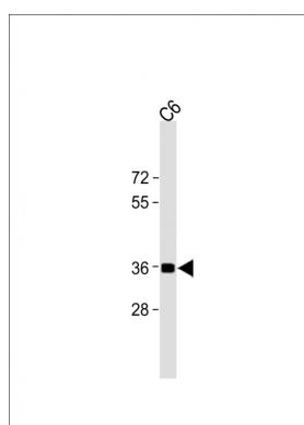
All lanes: Anti-GAPDH Antibody at 1:1000 dilution + C6 whole cell lysate Lysates/proteins at 20 µg per lane. Secondary Goat Anti-mouse IgG, (H+L), Peroxidase conjugated (ASP1613) at 1/15000 dilution. Observed band size: 36KDa Blocking/Dilution buffer: 5% NFDM/TBST.
